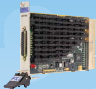
GX1164 1 \Omega to 64K \Omega programmable resistance, 1 \Omega resolution
