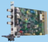
GTX2220 1.3 GHz Universal Time Interval Counter
