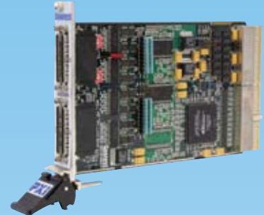
GX5281 High Speed Dynamic Digital I/O, 50 MHz data rate
