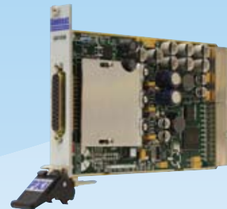
GX1838 Precision Multi-Channel DC Source (-10V to +32V)
